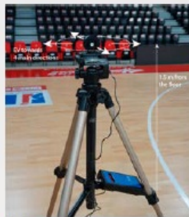
Mobile Cameras Illuminance (EV) Measurement
