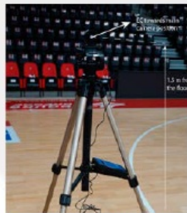
Main Camera Illuminance (EC) Measurement
