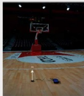
Horizontal Illuminance (EH) Measurement
