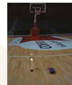
Horizontal Illuminance (EH) Measurement
